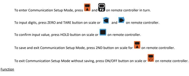
In Communication Setup Mode, user can change the scale's serial communication manner to meet the receiver's requirement, like communication on/off status, baud rate, scale communication address, signal output mode, etc.
